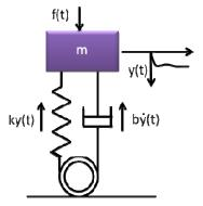
where k and b are spring constant and daming coefficient. Draw the free-body diagram and derive the ordinary differential equation of the shock-absorber dynamic model
